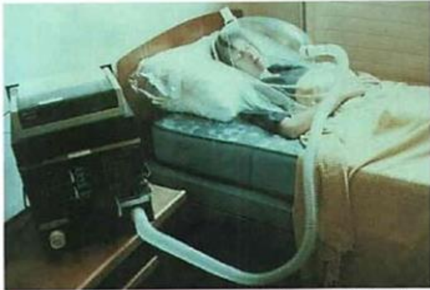
FIGURE 2-5 Measuring resting metabolic rate (RMR) using a ventilated hood system. (Courtesy The Dunn Nutrition Centre, University of Cambridge, Cambridge, England.)
